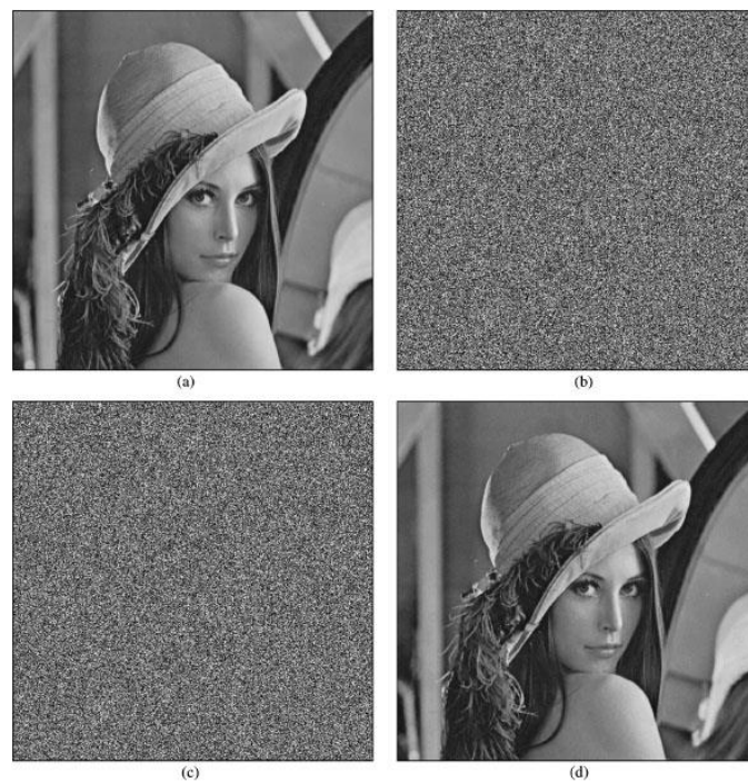
Fig 4 (a) Original Image converted into gray scale (b) Encrypted Image (c) Encrypted Image sent to Data Hider (d) Decrypted Image as well as Data
